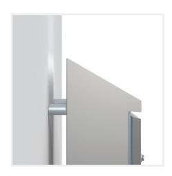
**Description:** Mounting brackets for hygienic wall fixing. Provides an space between the enclosure and the wall to facilitate cleaning operations. It includes the sealing washers to guarantee the IP rating. Machining required. Design according to EHEDG standards.
