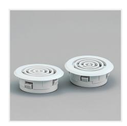
**Description:** For ventilating the enclosures. Can be concealed if mounted on the inside panel of the double walled corner. Machining is required (hole 34.9 mm diameter).
