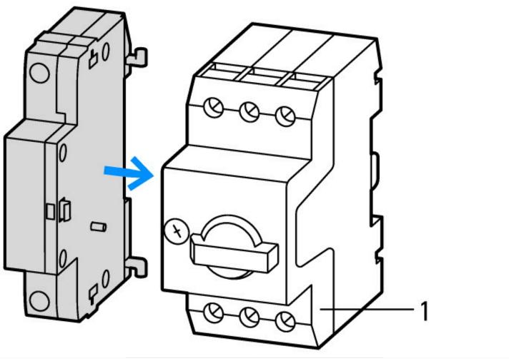
1: Motor-protective circuit-breakers
